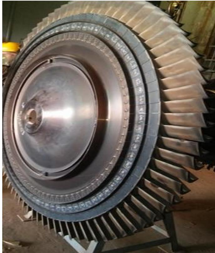
Figure I.15 : La roue HP (turbine MS5002B )
