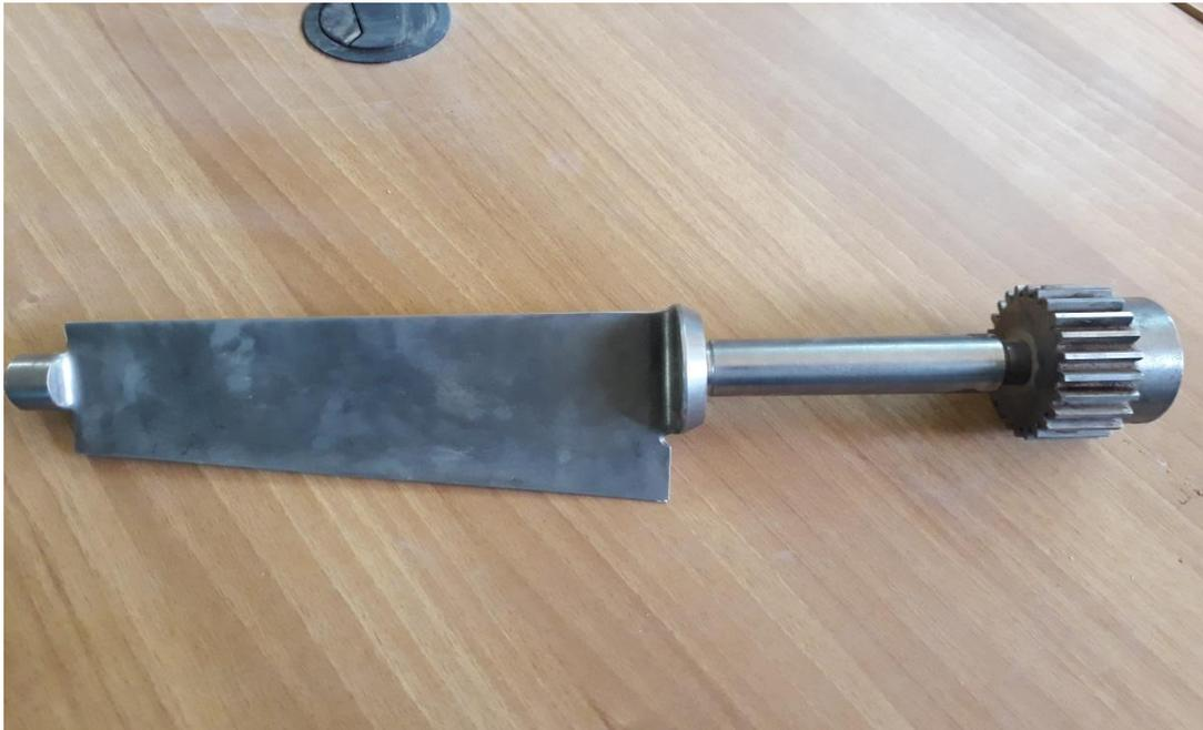
Figure I.3: Ailette IGV turbine MS5002B
