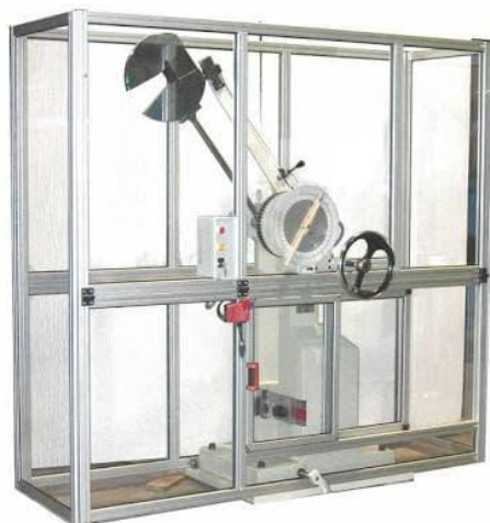
Figure II.26 - Photo du mouton de Charpy
