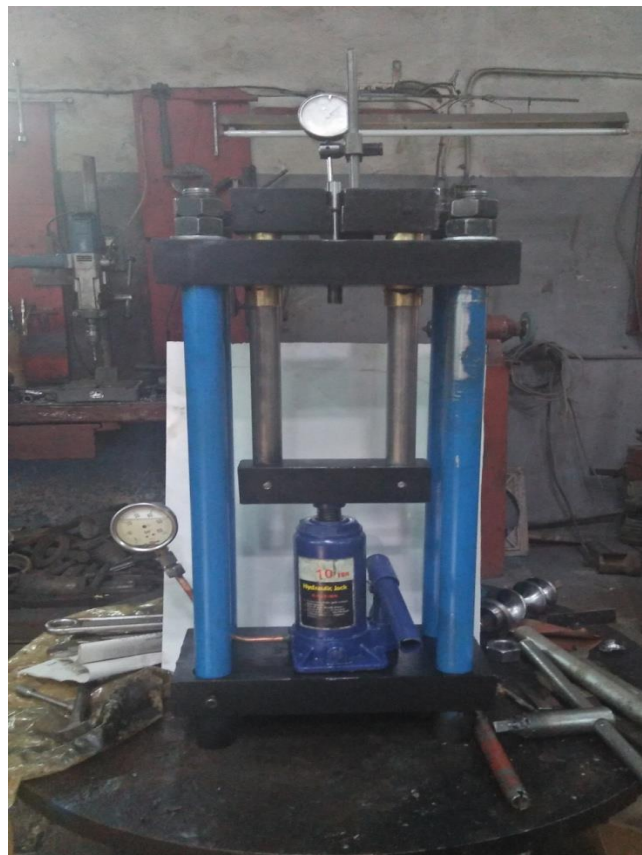
Figure (3.18) : machine de traction manuelle
