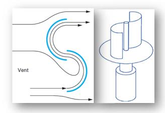
Figure I. 20: Éolienne type Savonius [6] [30].
