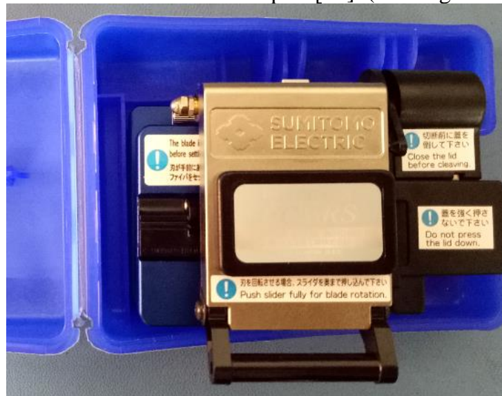
Figure III.19 : Cliveuse FC-6RS-C de Sumitomo
