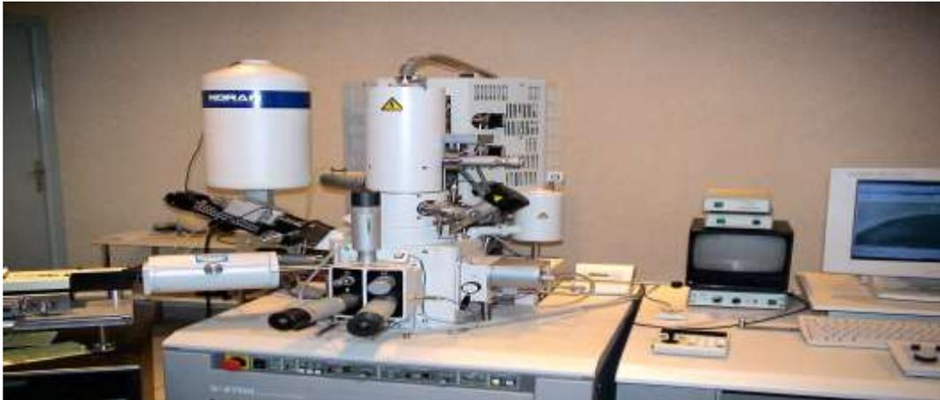
Figure III.15: MEB enmission de champ S4700 (SEM field emission S4700)<sup>15</sup>
