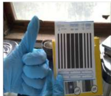
Figure 61: test Bowie-Dick conforme
