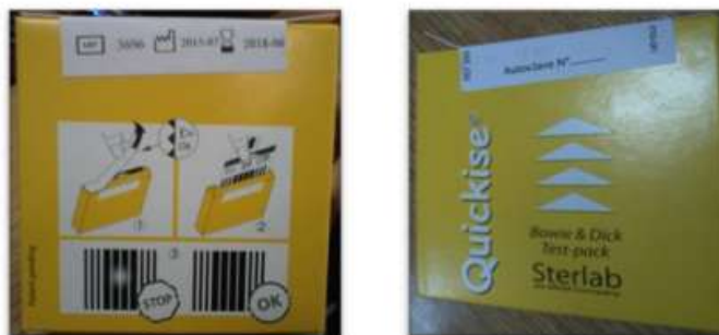
Figure 31: le paquet -test Bowie-Dick
