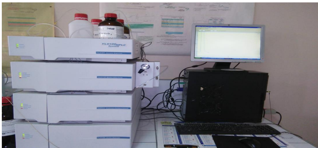
Figure 12 : Appareil HPLC YL9100.
