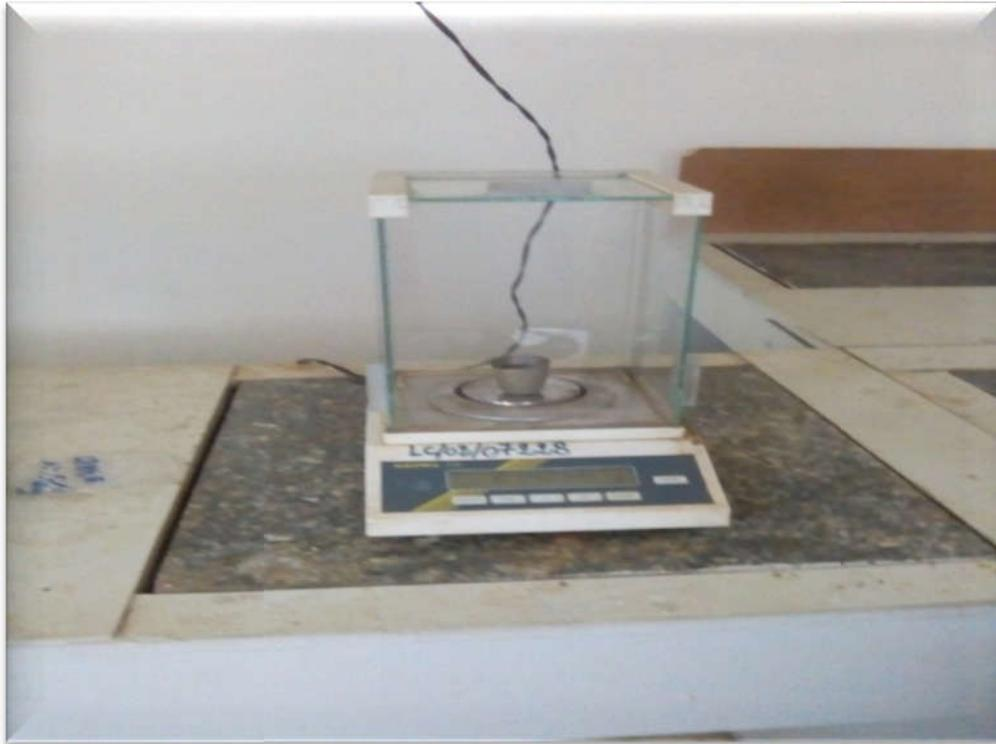
Figure IV.34: Balance analytique type KERN 770
