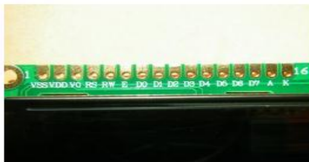
Figure III.4: Brochage d’écran LCD.
