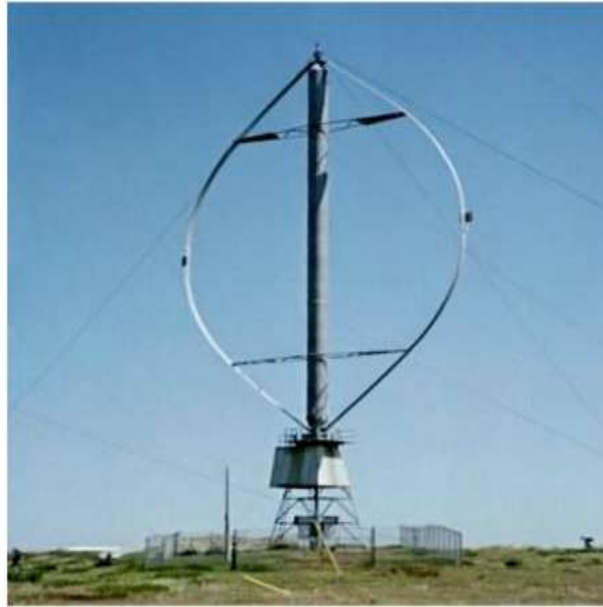
Figure 2-3. Eolienne de Darrieus [2]
