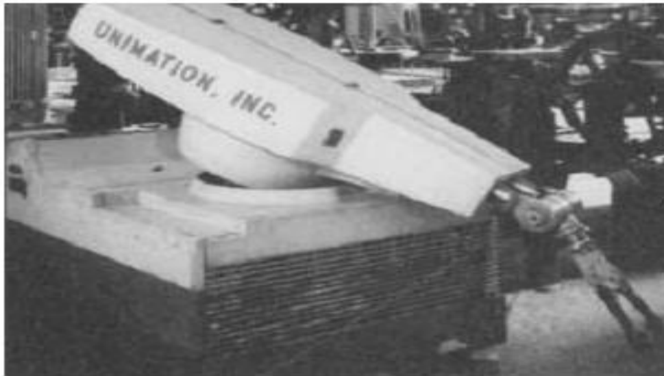
FIGURE 1.2 – Premier robot industriel ‘Unimate’[W7].
