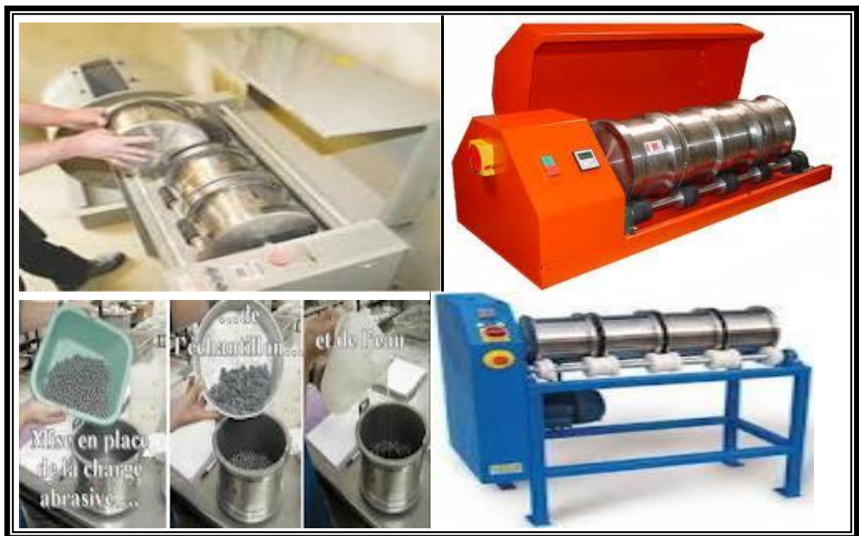
Figure 4.9 : Essai Micro Deval.
