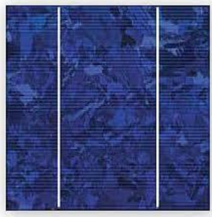
Figure (I.5) : le type de cellule poly cristalline
