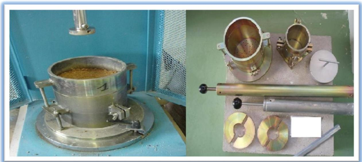
Figure 5. 5: Essai Proctor.[1]
