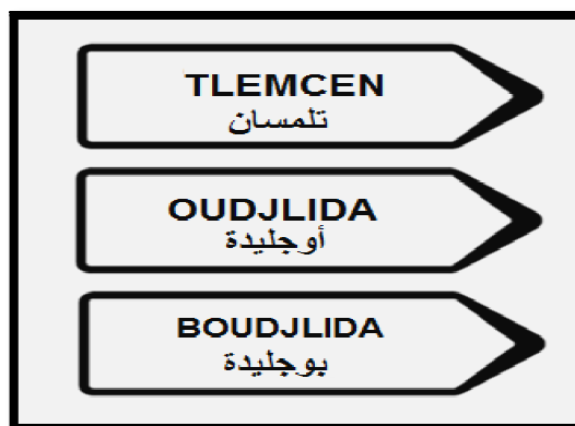
Figure 5.7: Signalisation de direction (type E4)
