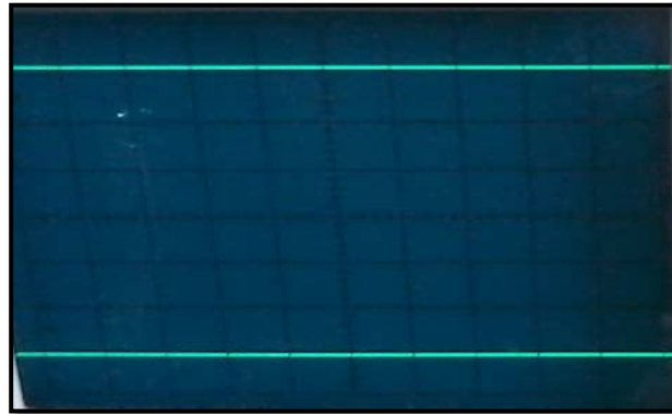
Figure 3.3 : Tensions continues +/-15 V de l'alimentation.
