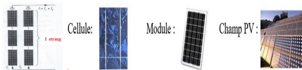
FIGURE II.1 – cellules, modules et champ panneaux photovoltaïques
