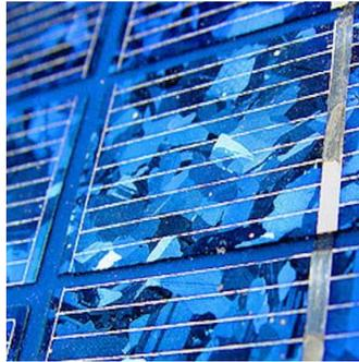
**Figure 9:**Cellule poly-cristalline [10]
