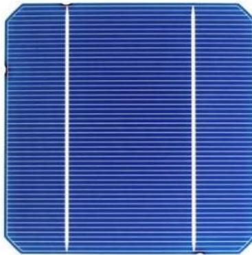
**Figure 8:**Cellule monocristalline [10]
