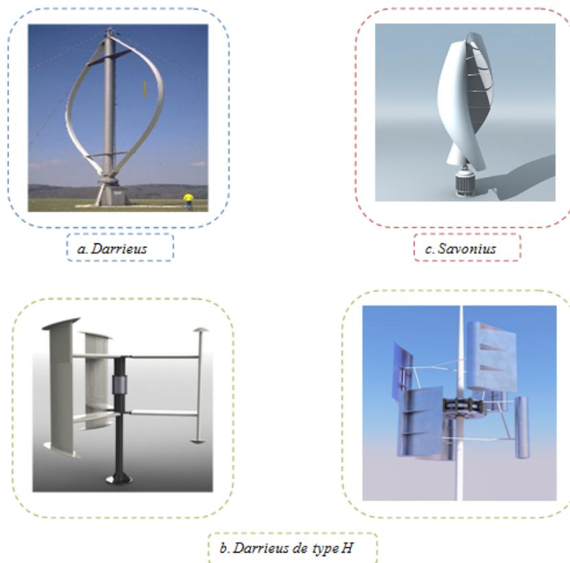
FIGURE I.2 – Exemples des constructions VAWT
