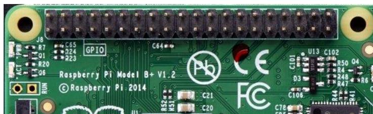
Figure 5 Interface GPIO de la Raspberry pi
