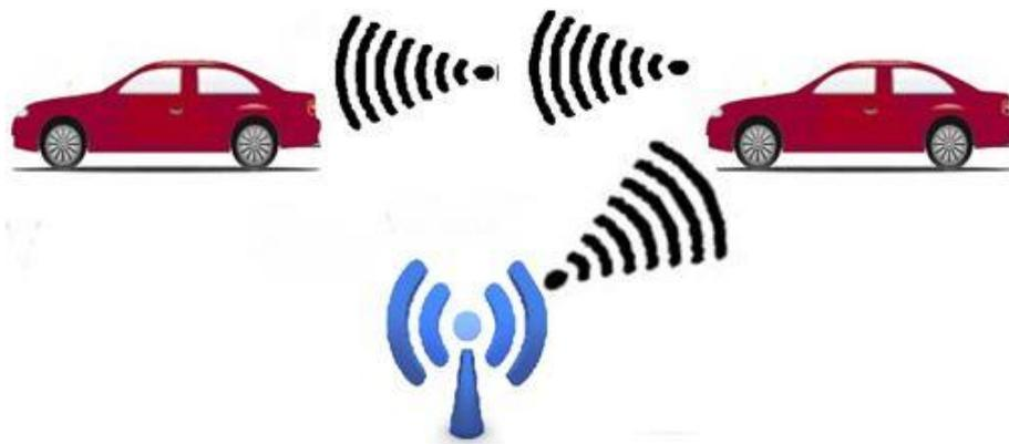
Figure 5 : Communication Hybride (V2I+V2V).
