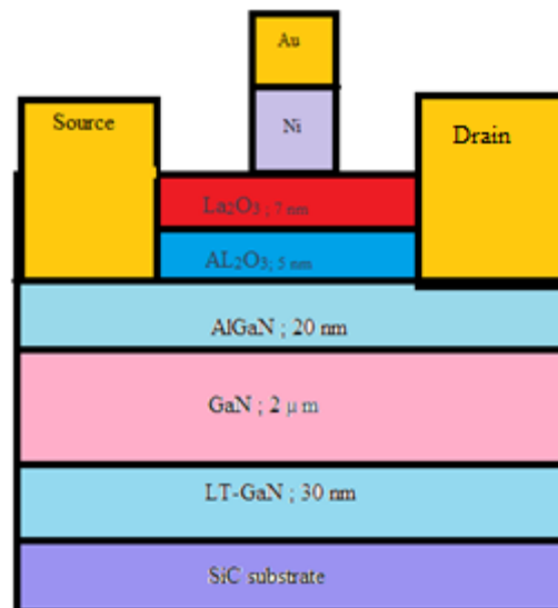
Figure III.3 : Topologie de la structure MOS-HEMT [28]
