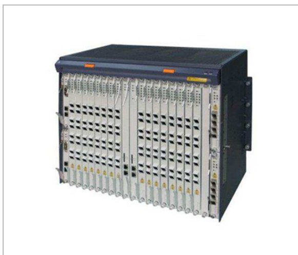
Figure II.22 : Exemple d'un MSAN ZTE [60]
