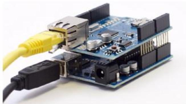
Figure III.5 Arduino UNO +shield Ethernet.
