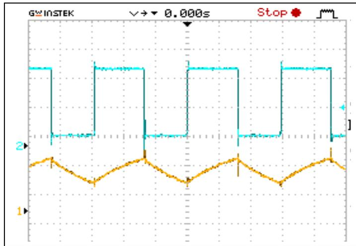
**FIGURE IV.7: SIGNAL CARRE DE (40KHZ) ET LE SIGNAL TRIANGULAIRE DE C1**
