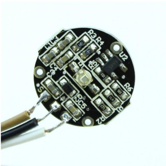
Figure 49 : circuit imprimé pulse sensor
