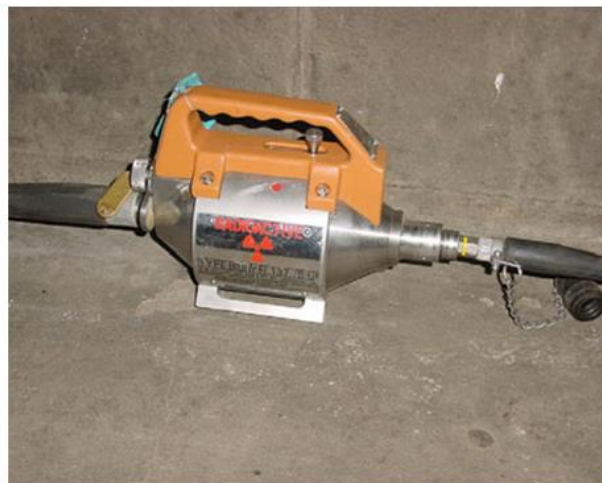
Figure 1.15 – Source d'Iridium 192 (Balayssac, 2012).
