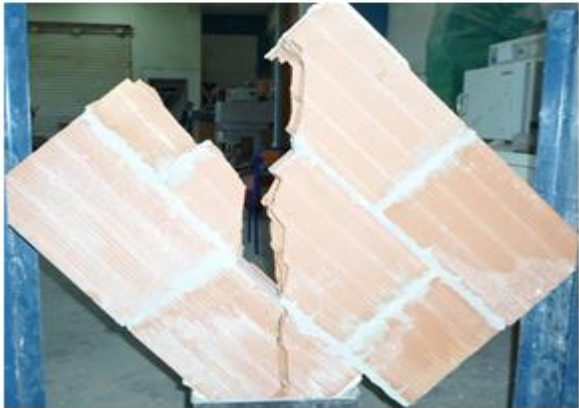
Figure 4.4: Rupture selon la diagonale.
